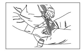
If the belt stops before it reaches the buckle, tilt the latch plate and keep pulling until you can buckle the belt.
